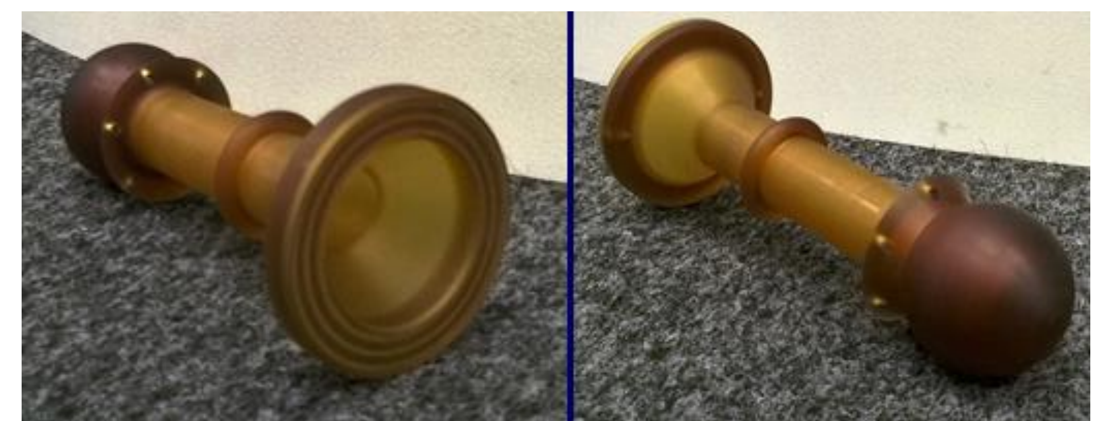
Nice Breast Applicator (NBA) ; Diameter between 3 and 5 cm (Ultem material)
