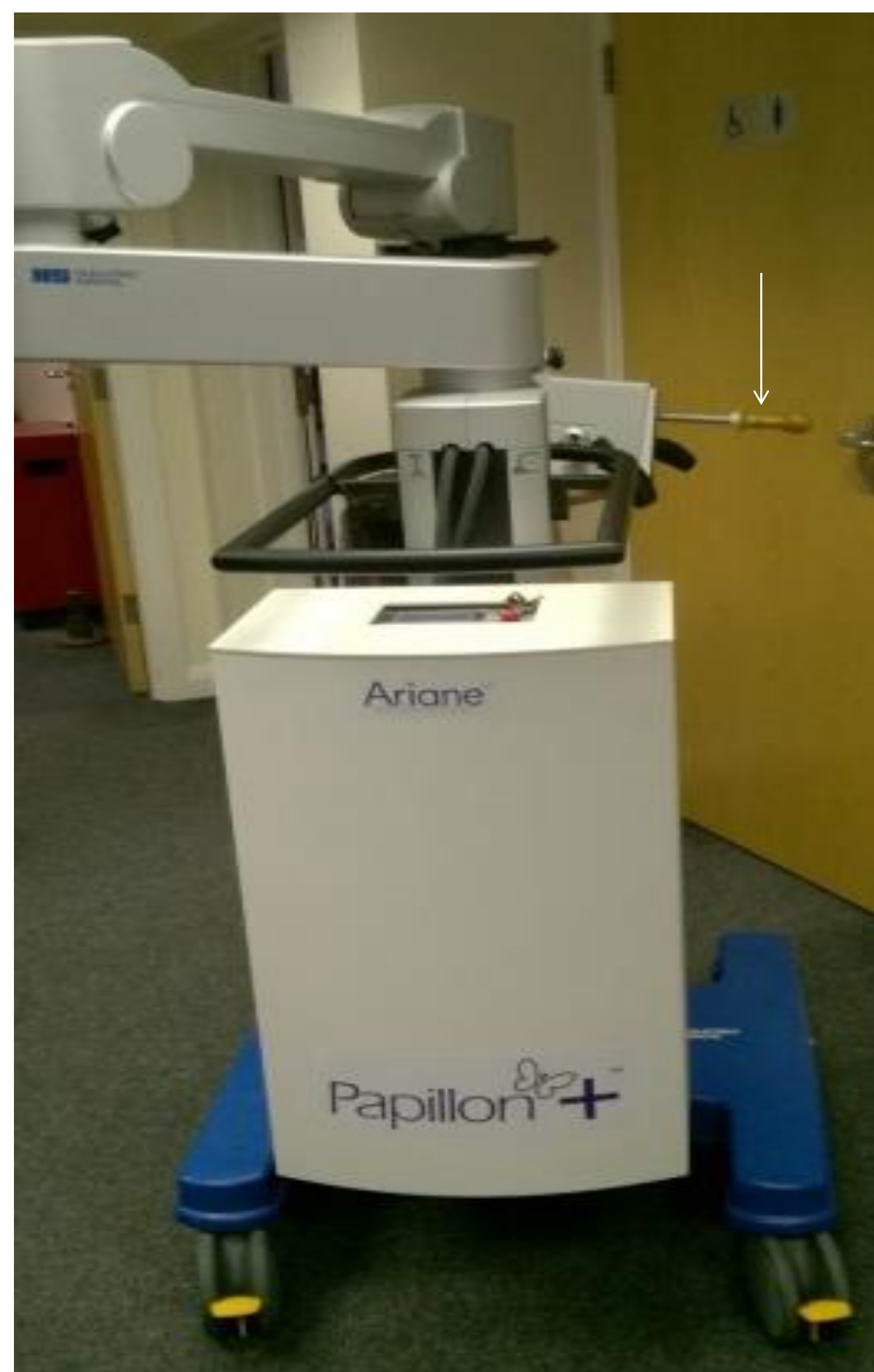
50 KVp x-ray generator. NBA applicator fixed on x-ray tube-rod (arrow)
