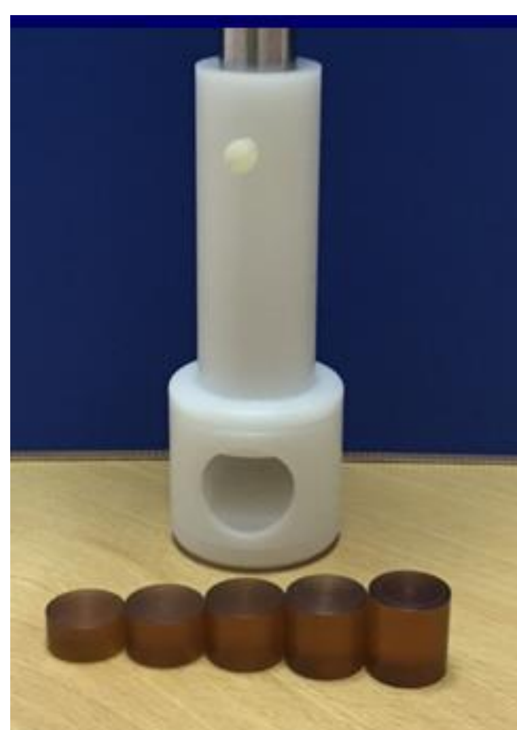
Dose quality control using a dedicated plastic insertion system and sham ultem applicators of different diameters mimicking the NBA spherical applicators.
